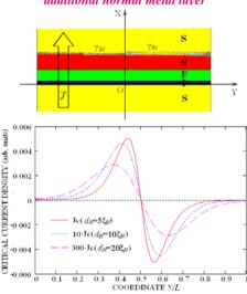
The critical current density distribution along the junction has the other scale, much longer than in SIFS. The scale depends on  $\xi_N$ . It is a consequence of the proximity effect. The junction length  $L=3000 \xi_R$
