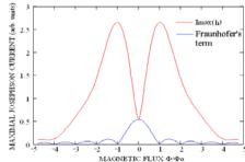
**Maximal Josephson current** through the junction (in the units of  $2\pi T/eR$ ) vs. the magnetic flux (in the units of  $\Phi_0$ ) in the vicinity of 0- $\pi$  transition
