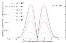
The junction critical current (in the units of  $\pi T/eR$ ) as a function of the external magnetic field near the point of 0- $\pi$  transition at various S/F boundary damping parameter  $\gamma_{B2}$ . Two different scales (small and extra large field).
