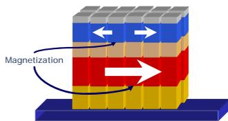
3. SiO<sub>2</sub> insulates the magnetic layers
