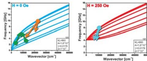
Fig. 3: For 0 Oe, all magnon splitting processes are allowed. At 250 Oe, spin wave emission below 4 GHz is forbidden.
