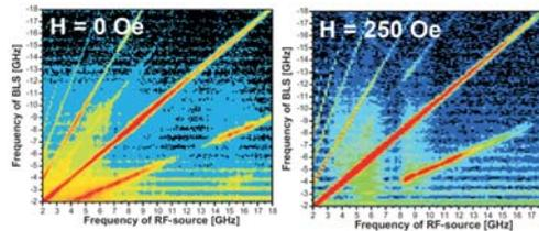
Fig2: Spectral intensity as function of 13dBm RF excitation frequencies for in-plane H = 0 Oe and H = 250 Oe magnetic fields.
