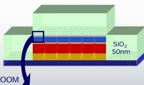
4. E-beam exposure defines 80 nm point contact and side contacts in PMMA resist.
