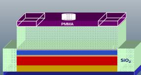
5. BHF dip etches a hole into the SiO<sub>2</sub> layer. Side contacts are opened. Resist strip is done afterwards with acetone and IPA
