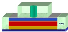
6. Unmasked sputter deposited Au/Ti film contacts the magnetic layers. Optical lithography defines CPW top electrodes. Second Au/Ti deposition is patterned by means of lift-off.
