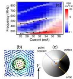
Fig. 5: (a) Experimental PSD and micromagnetic simulations at H = 350 mT (solid squares). (b), (c): Top view and in-plane component magnetization dynamics simulated for I = 30 mA.
