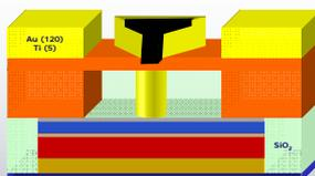
8. Ion milling transfers FOX12 pattern to CPW electrodes. Dry etching stopped when SiO<sub>2</sub> layer is reached.
