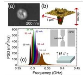
Fig. 4: (a), (b) SEM and AFM images of point contacts. (c) Low Frequency PSD at H = 210 mT (out-of-plane) for different applied DC currents.
