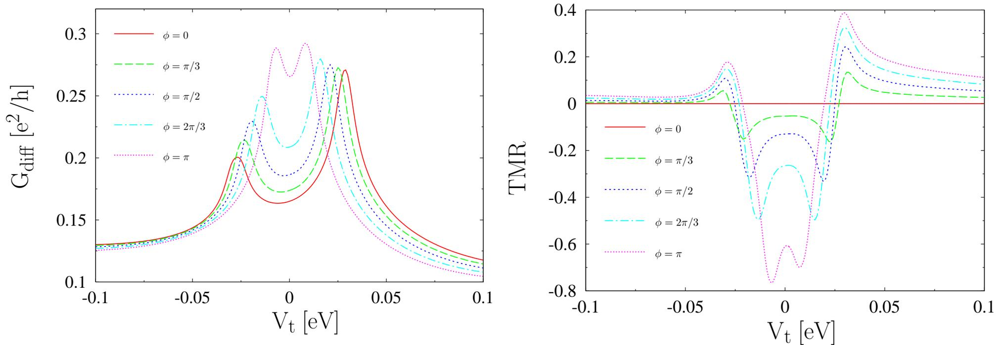
Figure 3: Differential conductance (left panel) and tunnel magnetoresistance  $\text{TMR} = [G_{\text{diff}}(\phi_L = 0, \phi_R = 0) - G_{\text{diff}}(\phi_L, \phi_R)] / [G_{\text{diff}}(\phi_L = 0, \phi_R = 0)]$  (right panel) calculated for parameters as in Fig.2 and for magnetic configurations as indicated in the figure.
