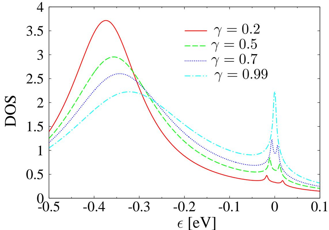
Figure 1: Density of states of the quantum dot attached to magnetic leads in antiparallel configuration, calculated for several asymmetry parameters  $\gamma$  as indicated in figure. The other parameters are:  $\epsilon_d = -0.45$  eV,  $U = 5$  eV,  $\Gamma_0 = 0.15$  eV,  $k_B T = 0.002$  eV,  $p_L = p_R = 0.2$  and electron band width extending from -25 eV to 25 eV.
