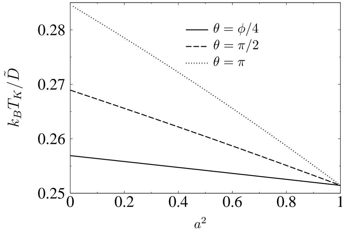
Figure 7: The Kondo temperature for QD asymmetrically coupled to leads vs.  $a^2 = (\gamma - 1)/(\gamma + 1)$  for several indicated magnetic configurations, the other parameters are  $p = 0.5$ ,  $\epsilon^d = -0.2$  eV,  $U = 5$  eV,  $D = 25$  eV.
