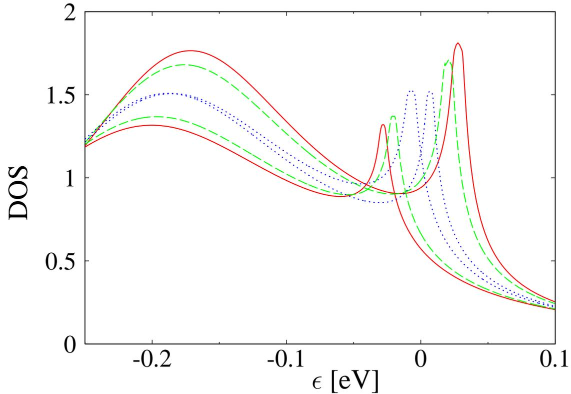
Figure 2: Density of states calculated for different magnetic configurations:  $\phi = 0$  (solid line),  $\phi = \pi/2$  (dashed line) and  $\phi = \pi$  (dotted line) and parameters:  $\gamma = 0.1$ ,  $\epsilon_d = -0.3$  eV,  $U = 5$  eV,  $\Gamma_0 = 0.2$  eV,  $k_B T = 0.001$  eV,  $p_L = 0.1$ ,  $p_R = 0.6$ , electron band width extending from -25 eV to 25 eV.
