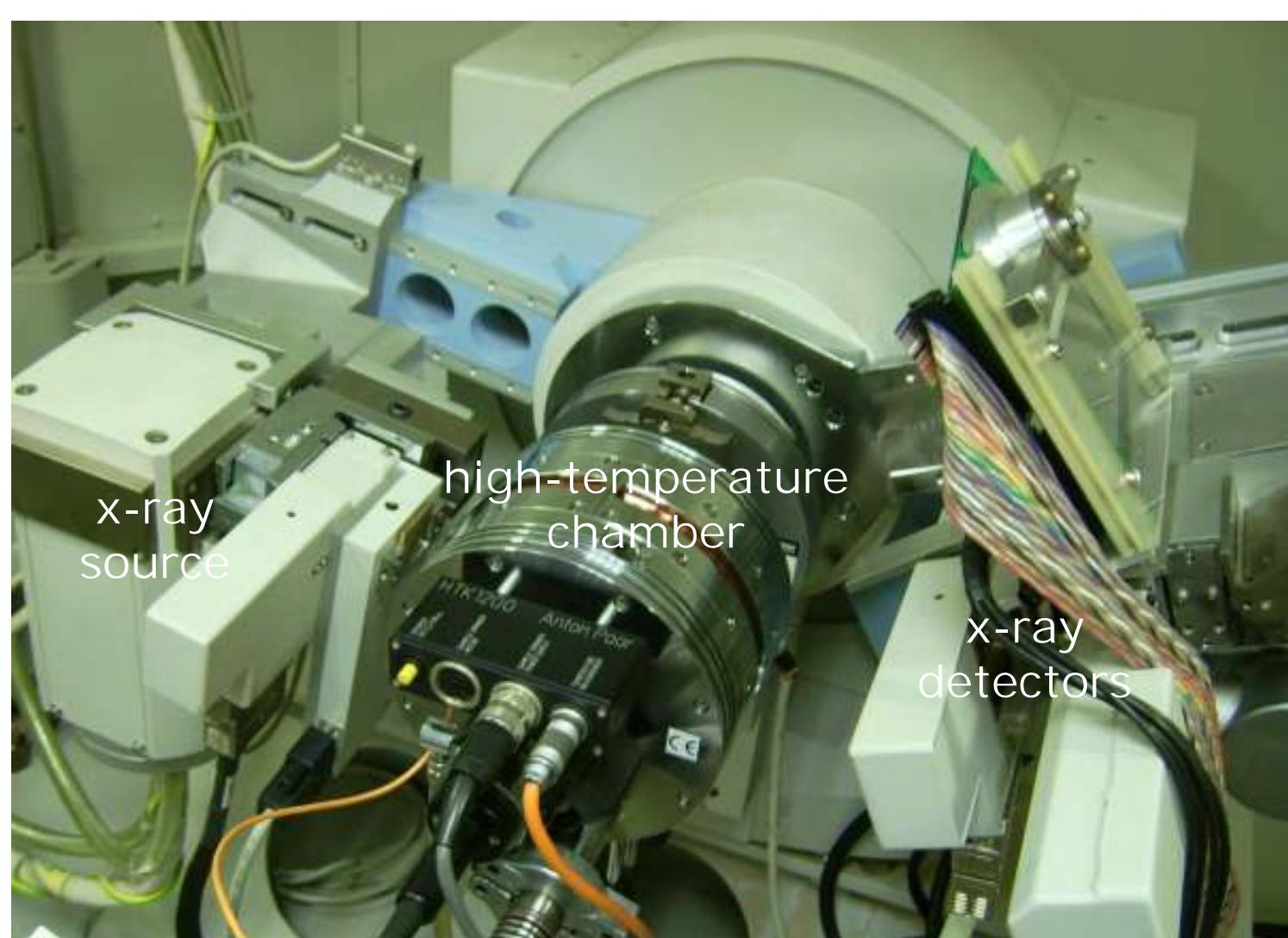
Samples were deposited by magnetron sputtering (Nordiko 2000 system). The films were characterized by X-ray diffraction using X'PertMPD diffractometer with Cu-anode. Surface roughnesses were measured by AFM. XRD -2 high-temperature in-situ measurements were performed using Anton-Paar HTK-1200 chamber.
